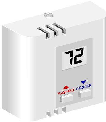
The Room Temperature Sensor (RTS) consists of a thermistor temperature sensor for monitoring room temperature, a Warmer and Cooler key provides limited adjustment of the setpoint temperature during normal occupied or comfort temperature setpoints.
