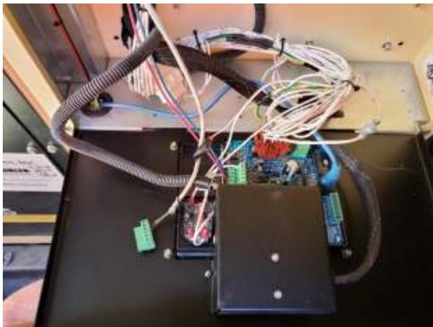
Figure 6 Rotate down the DEC3000 controller as shown.
