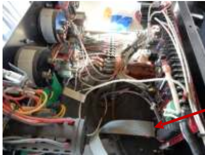
Figure 1 Main Control Board Annunciator and Communication board ribbon cable.
