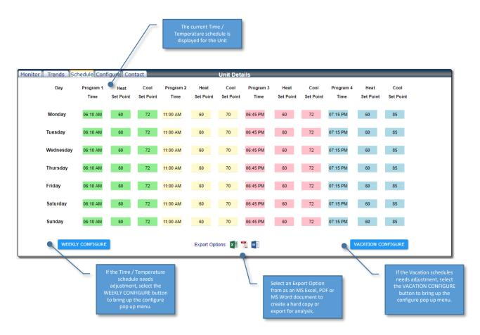
The ADRES control provide four time / temperature changes per day in the schedule and each day of the week can be unique. The ADRES control will run the HVAC unit to the above program schedule including any vacation schedule set while the unit is set to PROGRAM mode.
